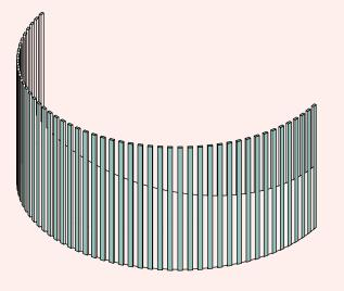
Subtraction Using the curve shape as a template cuts all top parts of those rectangular bars.
